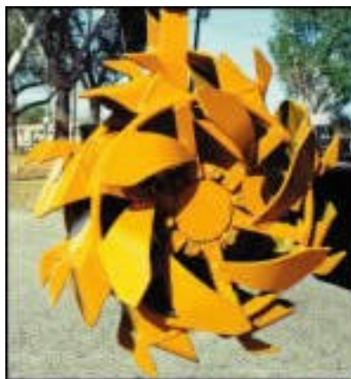
Figure 7.5 Dredge Head on a Hydraulic Cutterhead Dredge (Illustration Courtesy of Keene Engineering)
