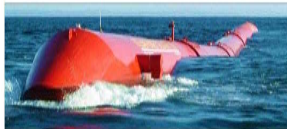
Attenuator Ocean Power Delivery Pelamis
