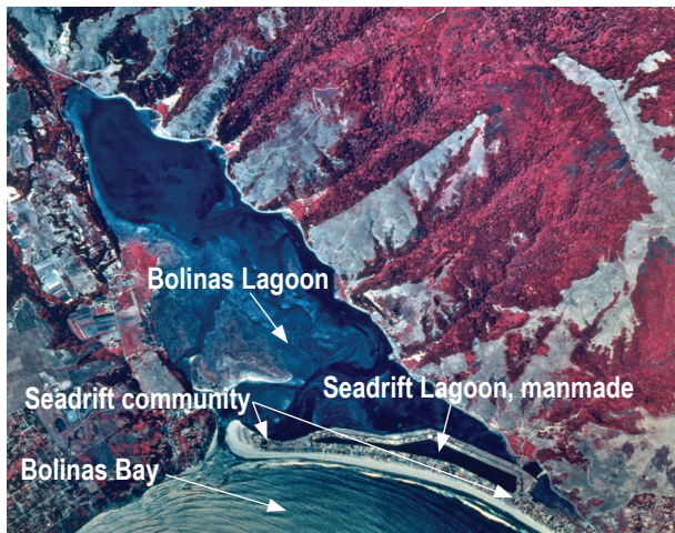
Figure 41. Aerial view of Bolinas Lagoon. The greatest change to Bolinas Lagoon has been the addition of fill to form the Seadrift community and artificial lagoon seen in the lower portion of the image.
